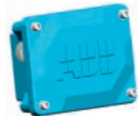
Auxiliary cast iron terminal box Frame size for motor sizes 160–250 (variant code 418): 111 x 162 mm, max. 18 strips. No earthing.
