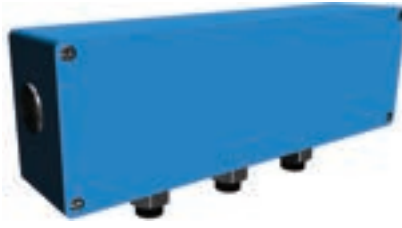
Large auxiliary aluminum terminal box for motor sizes 280–500. The size of terminal box ordered with these codes depends on the number of accessories ordered. 80 x 250 mm, max 30 strips. Earthing size M4
