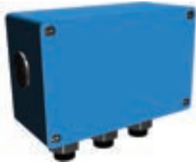
Small auxiliary aluminum terminal box for motor sizes 280–500 (variant codes 418, 568, 380, 569) The size of terminal box ordered with these codes depends on the number of accessories ordered. 80 x 125 mm, max 12 strips. Earthing size M4
